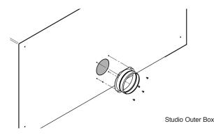
Thread the tube through the recess in the heat shield, and fit the flexible tube to the collar using the fixing band.
